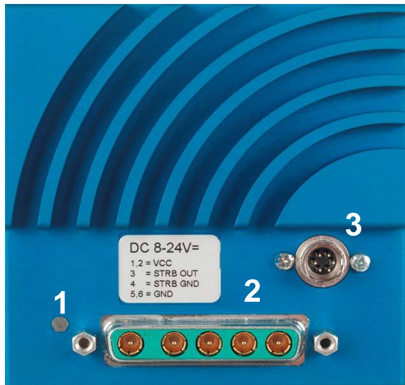
Image 3-2: CXP camera with 5W5 connector
